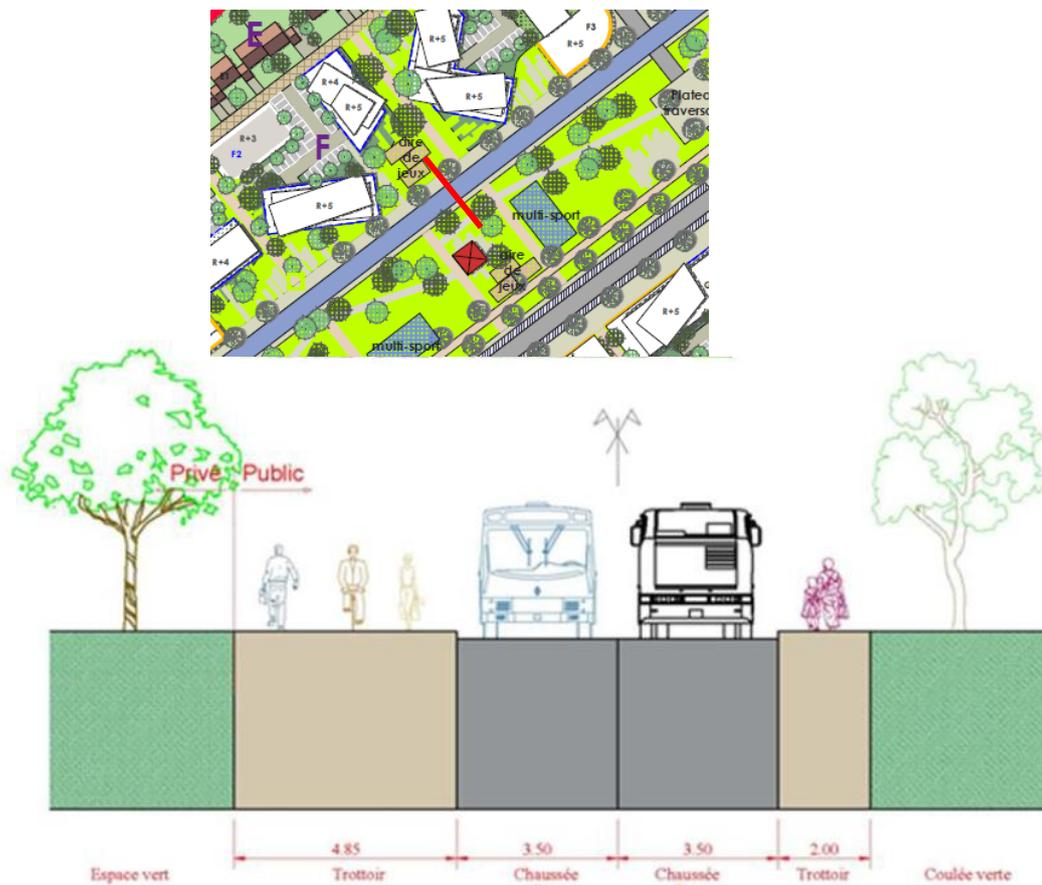
Figure 41 – COUPE DE PRINCIPE DE LA VOIE DE TRANSPORT EN SITE PROPRE – SOURCE : TPFI 2017
