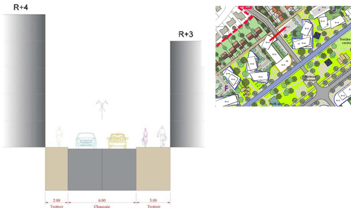
Figure 38 – COUPE DE PRINCIPE DES VOIES STRUCTURANTES SECONDAIRES – SOURCE : TPFI 2017
