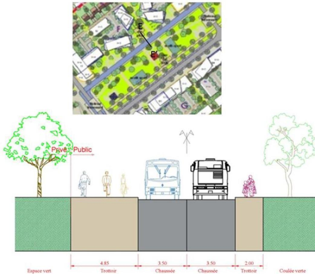
Figure 42 – COUPE DE PRINCIPE DE LA VOIE DE TRANSPORT EN SITE PROPRE – SOURCE : TPFI 2017
