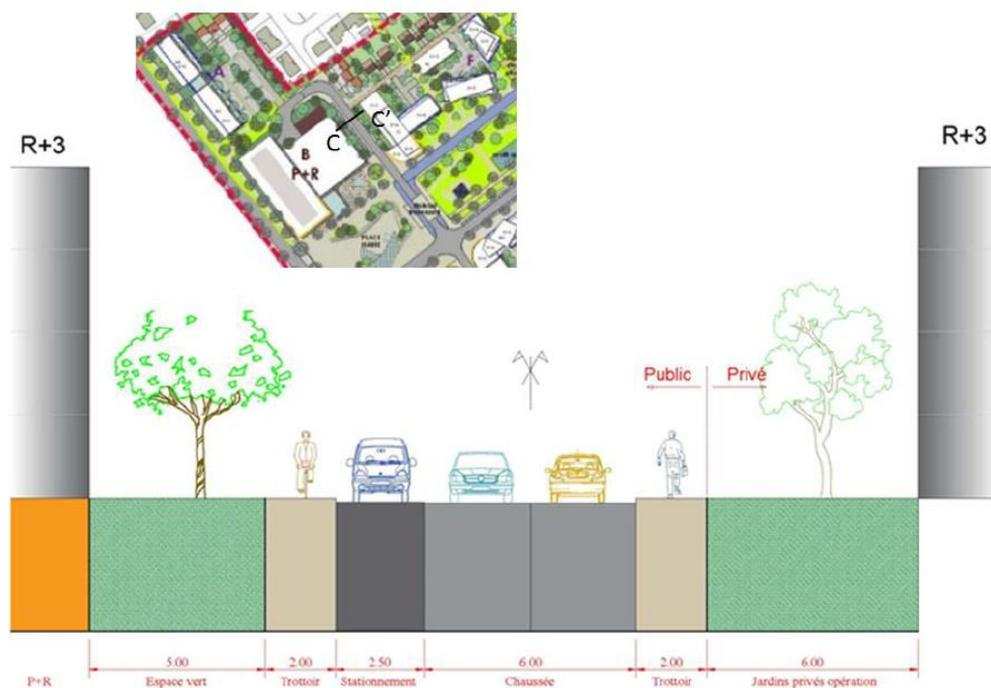
Figure 40 – COUPE DE PRINCIPE DE LA VOIE ALLANT AU TCSP – SOURCE : TPFI 2017
