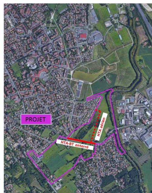
Figure 120 - CARTOGRAPHIE DES RESEAUX ELECTRIQUES - SOURCE : CITADIA 2017
