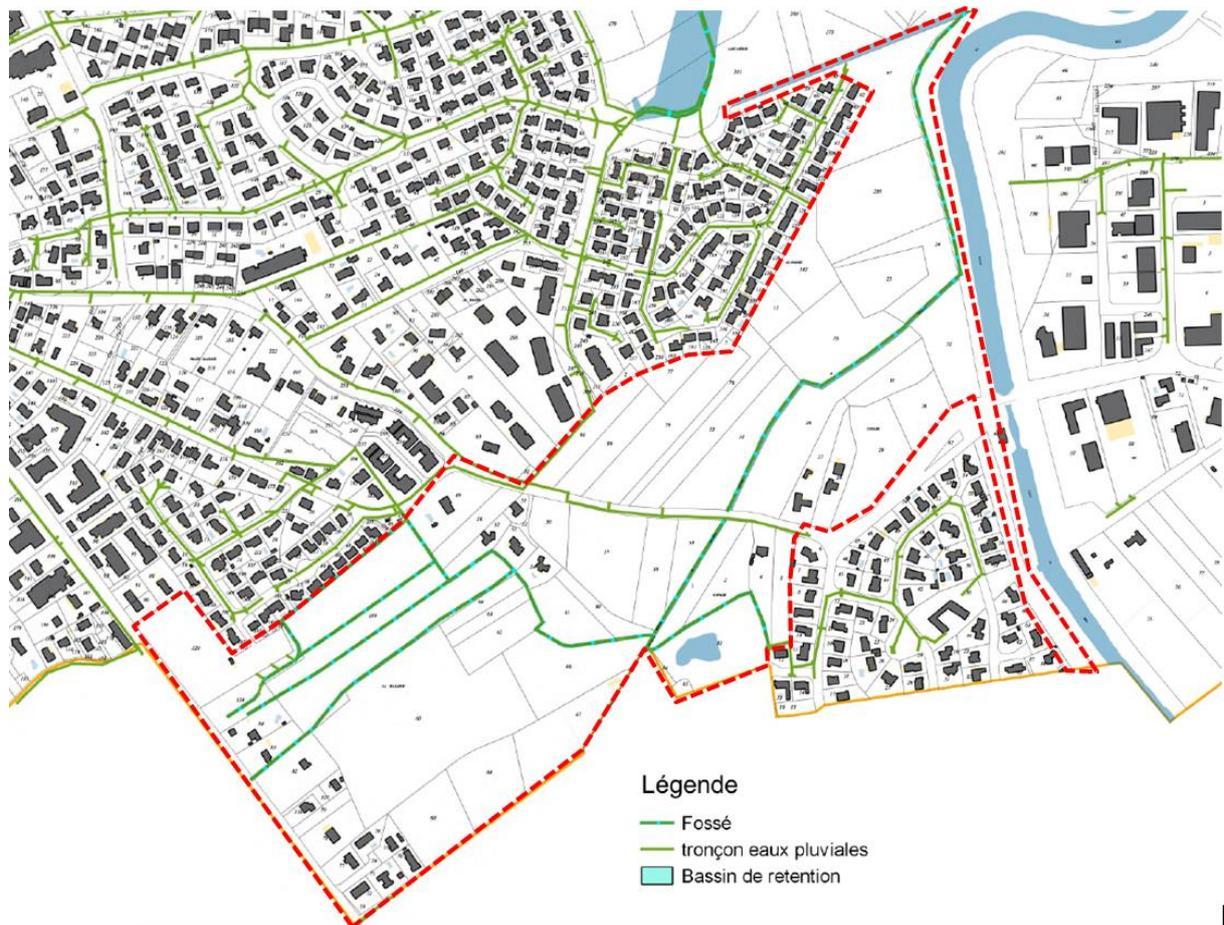
Figure 118 - CARTOGRAPHIE DES RESEAUX D'EAUX PLUVIALES 2017 – SOURCE : SICOVAL
